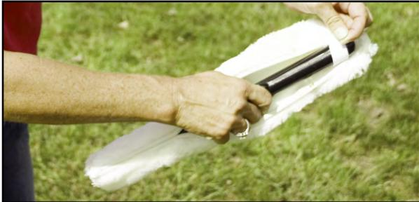
3) The ProCurve squeegee also comes fully assembled and ready to go. The 18" squeegee channel with rubber can be replaced by loosening the knob on the top of the handle and sliding it out. Slide the channel back into the ProCurve tool handle, center the channel, then secure the channel firmly by screwing the knob.
