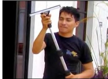
9) Squeegee the surface of the window or solar panel. **Be sure to angle the pole and squeegee handle to ensure that only the rubber is touching the glass surface.** You can squeegee from top to bottom, or side to side.
