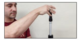
2) Insert the squeegee channel into one of the two included ProDesign handles by pressing on the lever underneath to open the jaw, slide the squeegee through the jaw until centered, be sure to have the side of the channel with the least amount of rubber showing facing down, release pressure on the lever to close the jaws.
