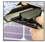
4) Insert the wash bar with sleeve attached onto the other ProDesign handle, slide the tab of the wash bar through the jaws until centered, release pressure on the lever to close the jaws.
